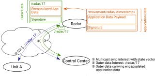
Fig. 3: Encapsulation of Application Data
