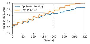
Fig. 7: Progression of successfully delivered data items over time, when comparing ER and SVS-PS.
