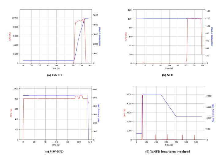
Figure 4: A sample of memory and CPU overhead of each forwarder when transferring a 1 GB file using ndnchunks using a fixed window (W = 100 packets). Note that file transfers in a-c do not start until approximately 60 seconds in to allow the producer to load the file into memory.
