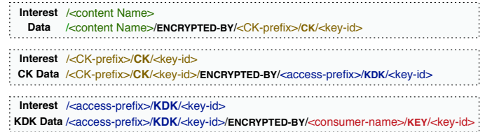
Fig. 5. Naming Convention in Name-based Access Control
