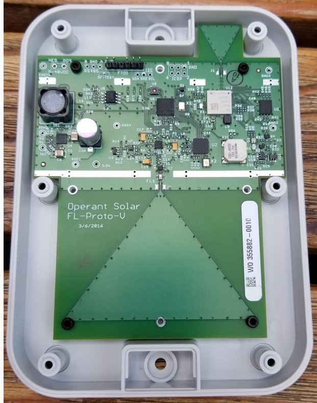
Figure 2.12: Operant Solar first generation Fleetlink prototype, running NDN-CCL.
