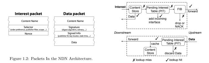
Figure 1.3: Forwarding Process at an NDN Node.
