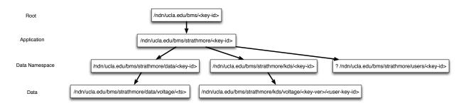
Figure 3.2: Relationship between data and key namespace (proposed).
