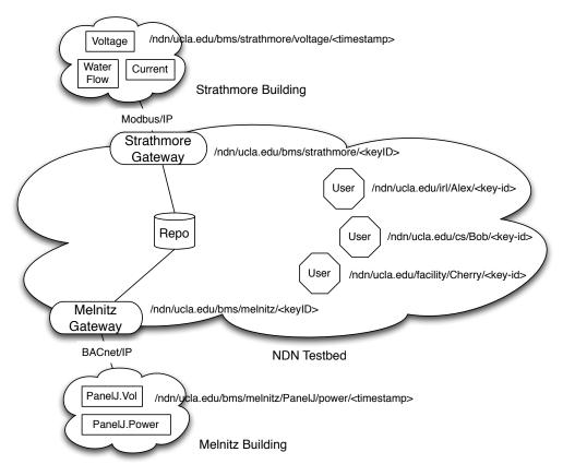
Figure 3.1: Building monitoring system architecture.
